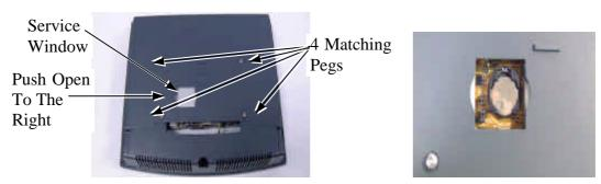
This battery socket requires a 3V button cell Lithium battery (CR2032) to support the system clock. The jumpers in this window are designated for COM port power supply and UPS battery detect functions. Please contact your dealer for technical support on setup of these jumpers. A new Lithium battery can support the system RTC for about 3 years. After the battery is nearly exhausted, the user must replace the battery otherwise the system RTC and system configuration setup will be lost.
